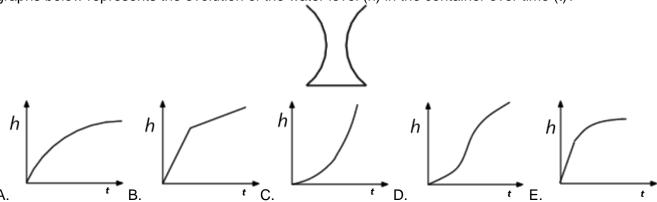
14. The water container below is filled with water at a constant rate of 1 liter per second. Which of the graphs below represents the evolution of the water level (h) in the container over time (t)?
