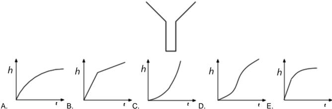
13. The water container below is filled with water at a constant rate of 1 liter per second. Which of the graphs below represents the evolution of the water level (h) in the container over time (t)?
