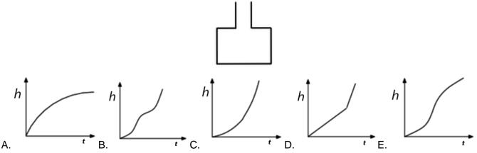
15. The water container below is filled with water at a constant rate of 1 liter per second. Which of the graphs below represents the evolution of the water level (h) in the container over time (t)?
